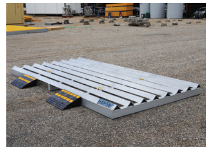
Rumble Grid on site
